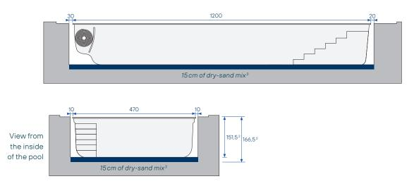
Note: the digging sizes do not take into account the necessary space for the coping stones.
